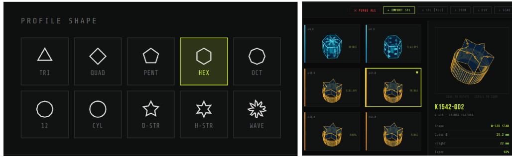
Fig. 2. First figure shows the profile shape options including triangle, diamond, pentagon, hexagon, octagon, and star configurations for tactile and visual distinction. Second figure shows ACCESS KNOB interface with a batch of 12 generated knob variants with hexagonal profiles. Parameters are displayed for the selected knob (K793-001) including shape, diameter, height, groove geometry, and bore specifications. The mutation engine enables rapid design exploration.
